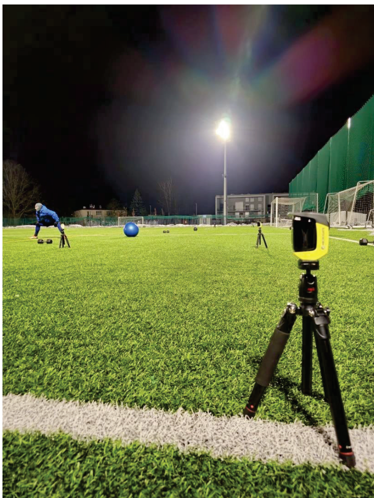
Figure 2. Microgate Witty System photocells are spaced at the measurement site.
