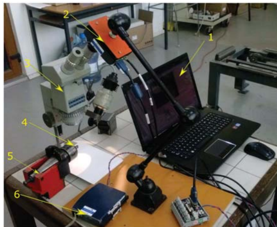
Figure 3. Image acquisition system for the automatic determination of tool wear.
