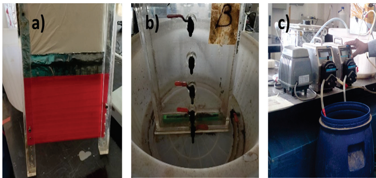
Figure 11. Photographs of the (a) membrane assembly, (b) bioreactor configuration, and (c) pilot-scale membrane bioreactor installation setup.
