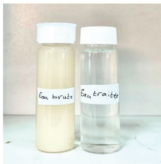
Figure 14. Soap effluent before and after coagulation–flocculation treatment.
