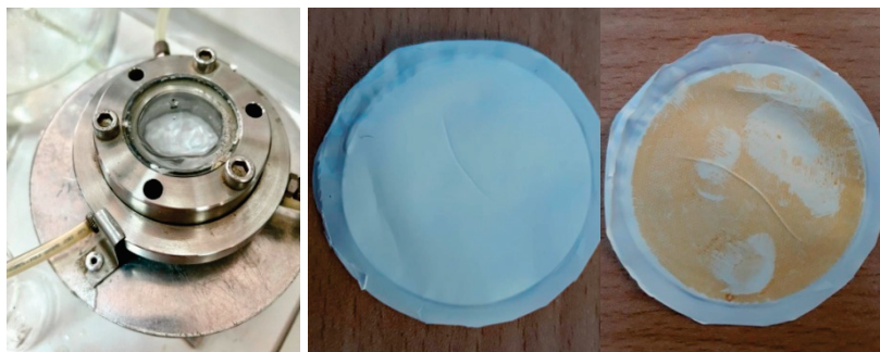
Figure 17. Ferric Chloride Residue on Membrane After Hybrid CF-MF Treatment.
