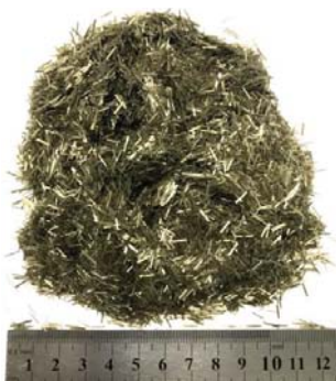
Figure 1. Morphology of basalt fiber with length of 6 mm in this study.
