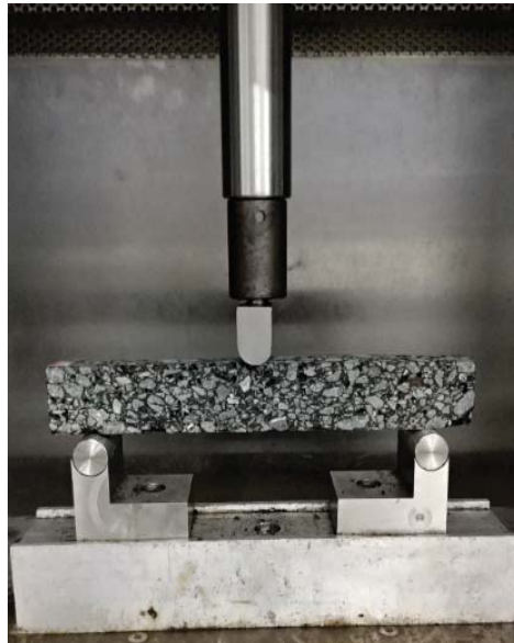
Figure 2. Three-points bending test set-up.
