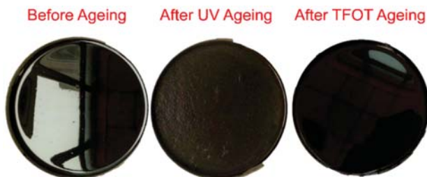
Figure 1. The plate with bitumen before and after ageing.
