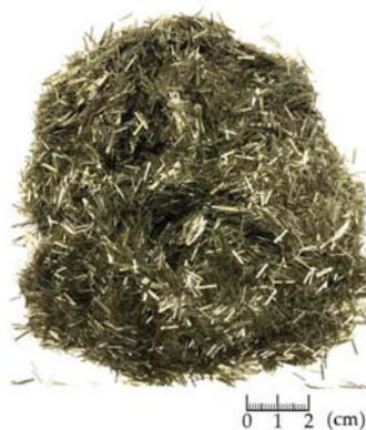
Figure 1. The golden-brown 6 mm long basalt fibers that were used in the study.
