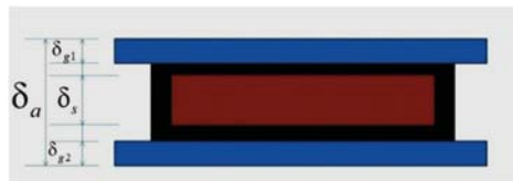
Figure 8. Schematic of asphalt film thickness measurement.
