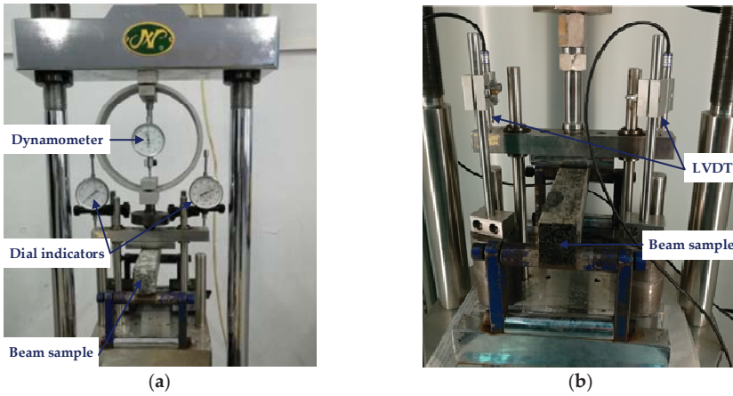
Figure 3. Low-temperature viscoelastic property tests: (a) Beam bending failure test; and, (b) Beam bending creep test.
