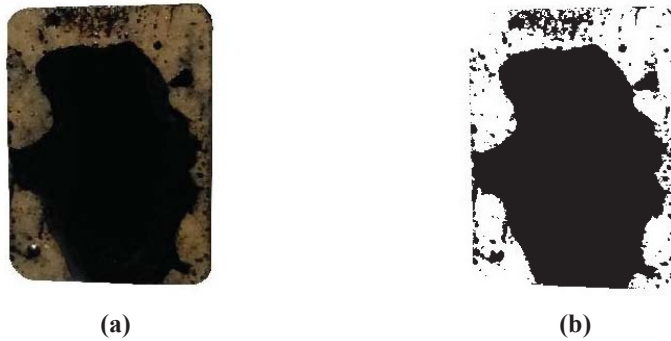
Figure 7. The image processing of test specimens with #110 asphalt and granite aggregate: (a) original image and (b) binary image.
