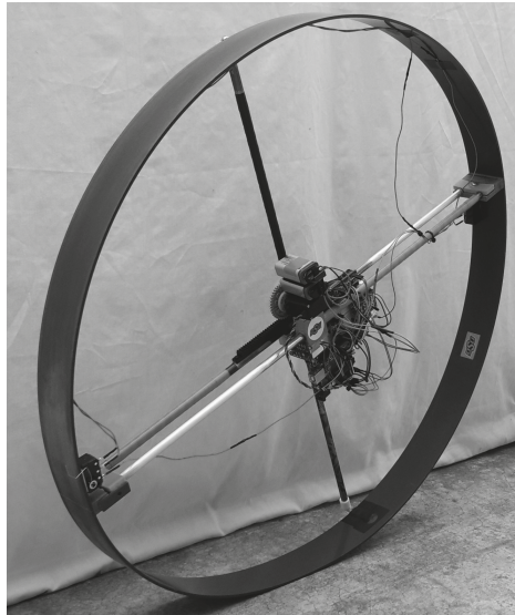
Figure 1. The OSU Roller has a mass of 0.950 kg with a perimeter of 2.095 m.
