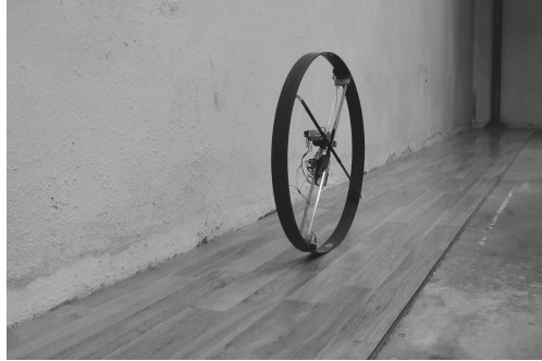
Figure 6. Roll track for the robot is a flat and level section of laminate flooring installed on concrete.
