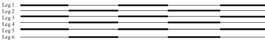
Figure 6. 3–3 gait diagram of 3-UPU hexapod walking robot.
