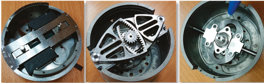
Figure 12. V2SOM prototype with each two functional blocks: (a) SAB: stiffness adjusting block, (b) SGB: stiffness generator block.
