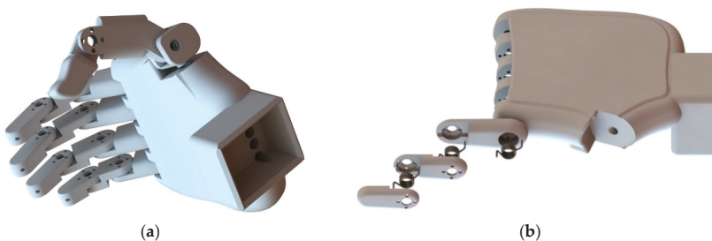
Figure 5. LARMBot 2 hand design: (a) Hand model; (b) Exploded view of a finger.
