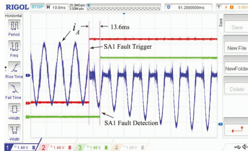
Figure 14. Input current and SA1 fault trigger and detection signals of phase A.
