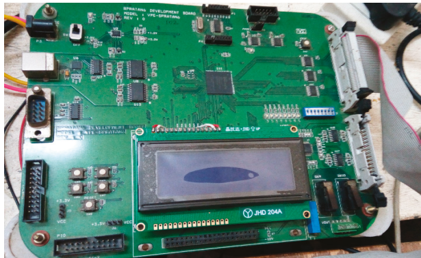
Figure 24. Xilinx Spartan6 development board.
