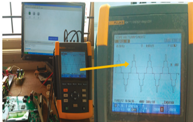
Figure 25. Seven-level stepped output voltage of TLBC-fed DCLCHB inverter system.
