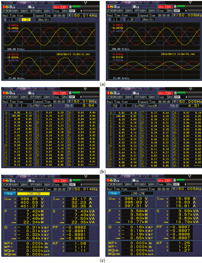
Figure 26. Snapshots of grid-side electrical quantities captured from the experimental set-up in Figure 1b by Hioki Power Analyzer PW3198 at P_o = 22 kW (left) and P_o = 11 kW (right): (a) line-to-line voltage and line current waveforms; (b) harmonic content of line current waveforms; and (c) output powers.
