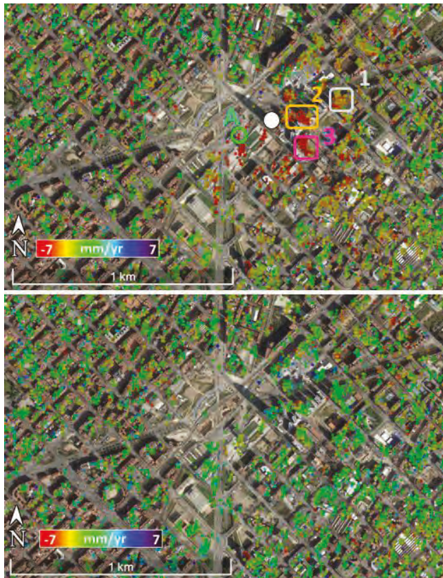
Figure 5. Examples of LOS accumulated deformation maps corresponding to the maximum of the displacement (12 April 2017, above) and to the recovery of the displacements (3 September 2017, below). In the above image, the three rectangles (grey-zone 1, orange-zone 2 and pink-zone 3) show the location of the three zones shown in Figure 6. The green circle A shows the location of the point considered in Figure 4. The white circle shows the location of the piezometer.
