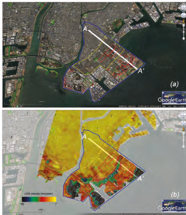
Figure 15. Subsidence rate map (2006–2010) generated with ALOS PALSAR data overlaid on a Google Earth image. The green polygons indicate the park area, red polygons indicate the location of high-rise buildings, the yellow polygon shows the highly populated residential area. The blue polygon indicates the border of Urayasu City and corresponds to the location of Figure 14a, and the A–A' line corresponds to the soil cross section in Figure 14a,b.
