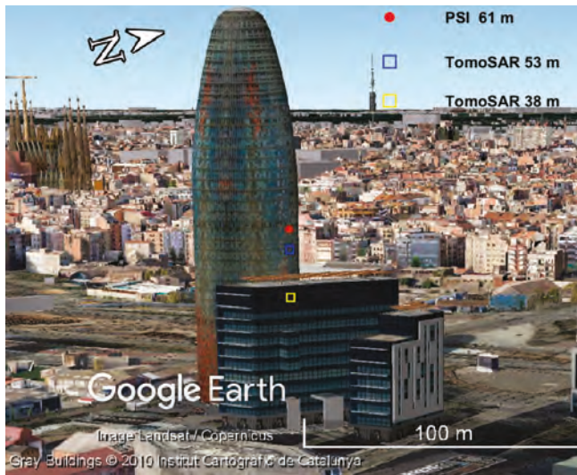
Figure 10. Difference in height estimate between TomoSAR and PSI in a common point.
