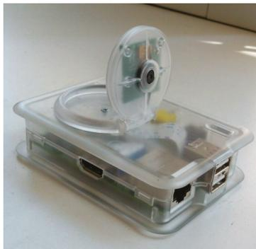
**Figure 2.** Image acquisition subsystem (Raspberry Pi 2 Model B and Pi camera), standalone configuration.
