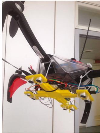
Figure 7. UDKS mounted on the UAV.
