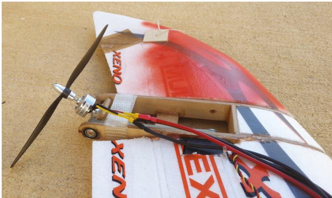
Figure 8. Tilt rotor mechanical structure.
