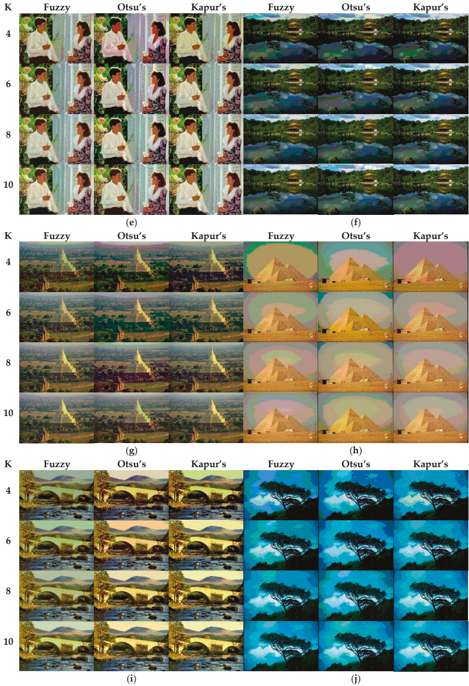
Figure 22. Segmented images at K = 4, 6, 8, 10 using CEFO algorithm based on fuzzy entropy, Otsu's and Kapur's entropy.
