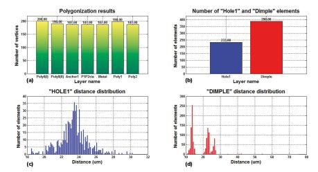
**Figure 11.** Sensor statistics provided by CMD, including (a) number of vertices for each fabrication technology layer; (b) number of "hole" and "dimple" elements included in the sensor structure; (c) distance distribution between "hole" elements; and (d) distance distribution between "dimple" elements.
