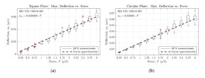
**Figure 15.** Experimental measurements of the sensor deflection versus a concentrated central force, assuming a AFM cantilever spring constant of  $k_{AFM}=42~\mathrm{N/m}$ . (a) For a square sensor; (b) for a circular sensor.
