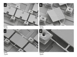
**Figure 4.** SEM pictures of alternative versions derived from the nominal design: (a) Butterfly-shaped pixel with longer rods; (b) Simple pixel without insulating legs; (c) H-shape pixel with thinner nanorods for enhancing the thermal insulation; rod-thickness = 30 nm; (d) Zoom of the legs (Figure 4c) attached to a stud that acts as a mechanical anchor and that provides electrical contact with the lines underneath.
