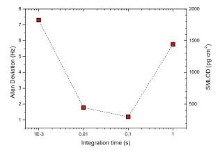
**Figure 7.** Allan deviation as a function of integration time measured in air conditions (atmospheric pressure and ambient temperature). The corresponding surface mass limit of detection (SMLOD) for each integration time is indicated in the right y-axis.
