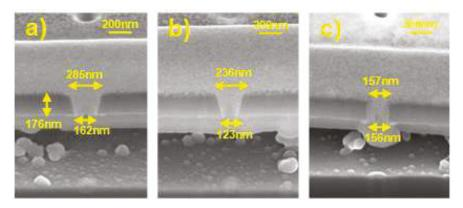
**Figure 3.** Cross-sectional scanning electron microscopy (SEM) images of etch holes with the variation of the beam current and target diameter of the focus ion beam (FIB) process. (a) Aspect ratio = 0.79 when beam current is 50 pA and target diameter is 160 nm; (b) Aspect ratio = 1.01 when beam current is 10 pA and target diameter is 160 nm. (c) Aspect ratio = 1.14 when beam current is 10 pA and target diameter is 80 nm.
