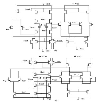
$\label{eq:Figure 7. (a) Input stage transconductance operational amplifier with common-mode feedback circuit (b) Gain booster V_n; and, (c) Gain booster V_p.$
