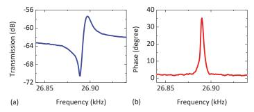
**Figure 5.** Electrical characterization results of the single-crystal SOI MEMS resonator. (a) Measured transmission (dB) and frequency response of the resonance; (b) Open-loop phase (degrees) around the first mode for  $V_{\rm DC}$  = 20 V and an input power of -10 dBm.
