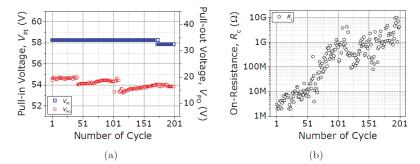
Figure 10. Evolution of (a)  $V_{PI}$ ,  $V_{PO}$  and (b)  $R_c$  over 200 switching cycles under vacuum conditions and  $V_{DS}$  fixed at 3 V. Compliance current limit is fixed to 1  $\mu$ A.
