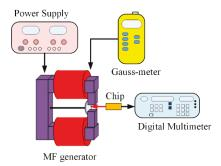
Figure 8. Experiment setup for the MMF sensor.
