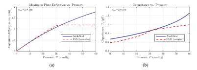
**Figure 12.** Comparison between the analytical and FEM models for circular MEMS pressure sensor with top plate radius of  $a_{top}=220~\mu m$ . (a) center deflection versus pressure response; (b) capacitance versus pressure response.
