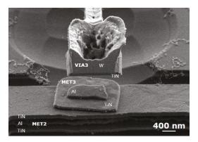
**Figure 6.** SEM image taken in the contact region of the seesaw relay showing the over-etch of the Al layer contained in the sandwiched MET3 layer of TiN-Al-TiN.
