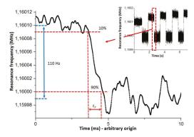
**Figure 9.** Resonance frequency according to the acquisition time. A 1 mW red laser is focalized onto the pixel under test (typical Figure 3c). Insert: Full data from our measurement of response time. The average frequency jump is estimated as 110 Hz. Then, the response time is extracted from one event fall time (red).
