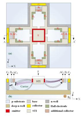
**Figure 1.** Micro magnetic field (MMF) sensor: (a) schematic structure; (b) cross-sectional view along line AA'. STI, shallow trench isolation; E, emitter.
