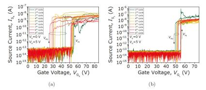
**Figure 5.** First nine current voltage (*I-V*) switching characteristics in ambient conditions of the (**a**) left and (**b**) right drain electrodes for the seesaw relay Type I (TiN-TiN contact).
