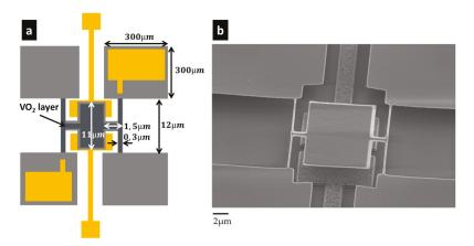
Figure 11. Torsional resonator design: (a) Schematics of the design; (b) SEM image of a typical pixel with a  $VO_2$  layer on top of both the plate and torsional rods, plus partially on the insulation legs.
