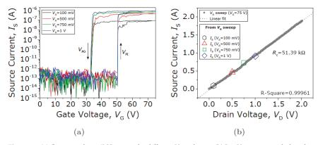
**Figure 14.** (a) Current voltage (I-V) curves for different  $V_D$  voltages. (b)  $I_{DS}$ - $V_{DS}$  sweep with the relay in its ON-state ( $V_G$  = 75 V), showing an ohmic dependence. The  $R_C$  values extracted from the I-V curves in (a) are also plotted (symbols).
