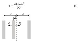
Figure 2. Differential capacitance model of the sensitive element.
