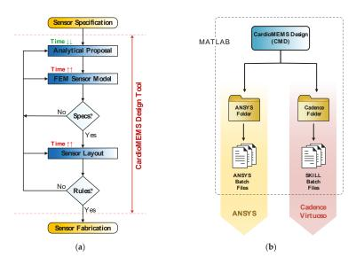
**Figure 9.** CardioMEMS Design (CMD) functionalities overview. **(a)** MEMS sensor design flow, highlighting those stages covered by CMD; **(b)** CMD output folders generated to export the designed sensor to ANSYS and Cadence Virtuoso.
