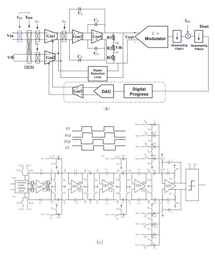
**Figure 3.** (a) Tunneling magnetic resistance-type sensitive structure, the physical printed circuit board (PCB) diagram is underneath the blue arrow (b) Three-axis digital tunneling magnetic resistance-type (TMR) sensor interface circuit System block diagram, the closed-loop feedback control of digital progress is shown in the dotted box (c) The fully differential 4th-order Sigma-Delta modulator.
