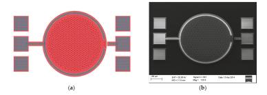
**Figure 13.** Final design stages for a circular MEMS pressure sensor with top plate radius of  $a_{top} = 220 \, \mu \text{m}$ . (a) Cadence Virtuoso layout view, generated through the SKILL batch files provided by CMD; (b) scanning Electron Microscope (SEM) picture of the fabricated sensor.
