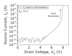
Figure 13. Current versus drain voltage curve in pull-in conditions to produce the initial native oxide breakdown (roughly at  $V_{DS} = 8 \text{ V}$ ).
