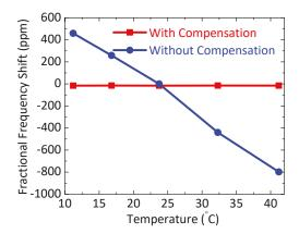
Figure 10. Fractional frequency shift (in ppm) as the device temperature is varied, measured from both the temperature-compensated and uncompensated oscillators over a temperature range of 10 to  $45\,^{\circ}\text{C}$ .
