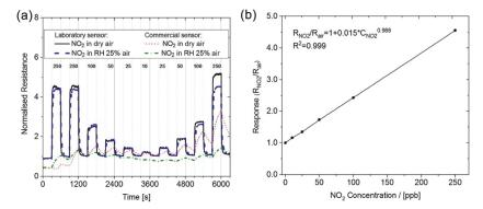
Figure 2. (a) The response of a laboratory  $WO_3$  based gas sensor and commercial MOX sensor with respect to  $NO_2$  in dry and humid air (b) response of the laboratory sensor as a function of  $NO_2$  concentration (from [33]).
