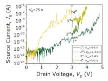
**Figure 11.** Successive source current versus drain voltage ( $I_{DS}$ - $V_{DS}$ ) sweeps showing the restoring of the contact performance after breaking down the grown native oxide on the W contact site of the relay.  $V_{GS}$  is fixed to 75 V to keep the relay in the ON-state.
