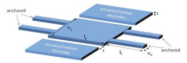
Figure 1. Schematic showing resonator dimension parameters.
