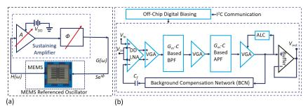
**Figure 3.** (a) Simplified system diagram illustrating the integration of the MEMS resonator chip with the CMOS sustaining amplifier chip; (b) Simplified block diagram of the programmable single-chip CMOS sustaining amplifier (corresponding to the same color-coded dashed-line box in (a)).
