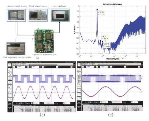
**Figure 8.** (a) The testing system of Sigma-Delta modulator Application Specific Integrated Circuit (ASIC); (b) The PSD of Sigma-Delta modulator; (c) The transient response of Sigma-Delta modulator; and, (d) Transient response after local amplification.
