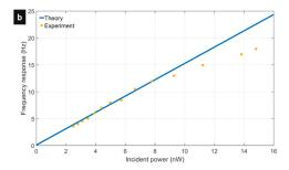
**Figure 8.** Measurement of the thermal response: (a) Resonance frequency shift induced by incident IR pulses (peaks of 17 nW); (b) Frequency shift when the incident power is varied from 2 to 16 nW.
