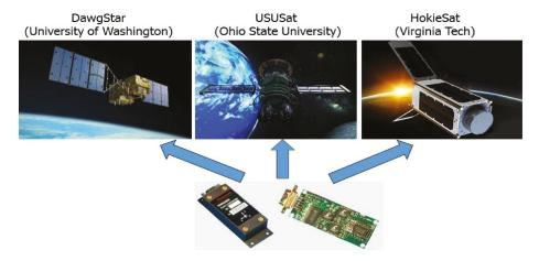
Figure 2. The HMR2300 magnetometer in Nano-satellite field.
