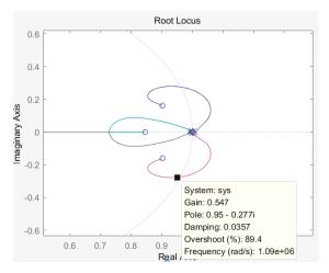
Figure 7. Root locus of the Sigma-Delta modulator.
