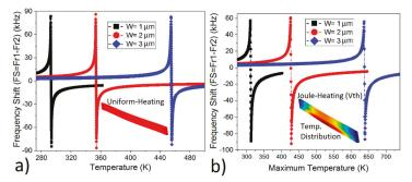
Figure 3. Frequency Shift (FS) with respect to 1 Kelvin (K) change by (a) Equation (1), and (b) COMSOL, when thickness (W) changes from 1  $\mu$ m to 3  $\mu$ m for Device 1 with a device length of 120  $\mu$ m.
