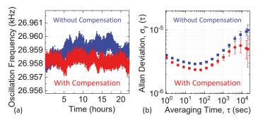
**Figure 9.** (a) Instantaneous frequency of the uncompensated and compensated oscillators over 24 h; (b) Measured Allan deviation  $\sigma_{\rm A}$  ( $\tau$ ) with and without real-time temperature compensation.
