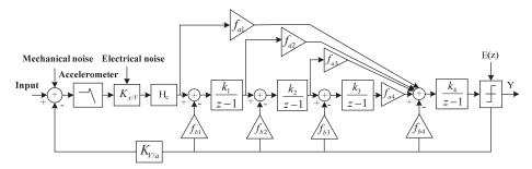
**Figure 6.** Analytical model of  $\Sigma\Delta$  micro-accelerometers.
