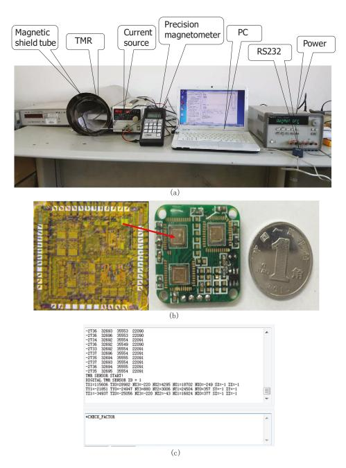
**Figure 10.** (a) The test platform of the three-axis digital magnetic sensor system (b) The photograph of printed circuit board (PCB) and ASIC chip (c) The data collection by RS232 in PC.
