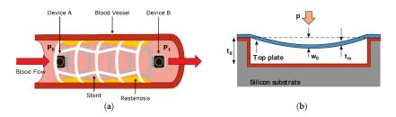
**Figure 2.** Building parts of a passive pressure sensing iStent. (a) Lateral view of the iStent implanted inside a blood vessel; (b) cross-sectional view of a MEMS capacitive pressure sensor.
