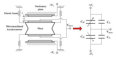
Figure 1. Vacuum-packaged bulk micro-accelerometer and equivalent bridge model.
