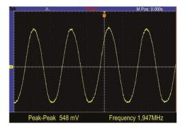
**Figure 6.** Time-domain oscillator output signal measured for  $V_{\rm dc}$  = 27 V.
