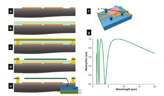
Figure 2. Synopsis of the fabrication process along the cross section AA': (a) Deposition of a 300 nm thick AlCu layer on a silicon substrate/strip lines/reflector wet etching; (b) 2  $\mu$ m deposition of a polyimide layer; (c) Etching of the polyimide layer to build up the metal studs, and deposition of the plate material; (d) Definition of the plate; (e) Dry etching O<sub>2</sub> plasma release; (f) 3D artist view of a pixel; (g) Absorption spectrum of the 2  $\mu$ m thick micro cavity.
