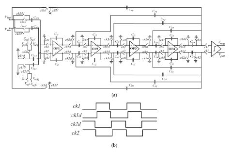
**Figure 5.** (a) High-order  $\Sigma\Delta$  modulator circuit; (b) the timing diagram of  $\Sigma\Delta$  modulator circuit.
