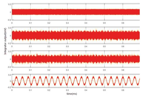
Figure 8. Output waves of each stage of the integrator.
