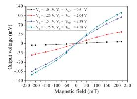
Figure 9. Measured output voltage in the y-direction MF.
