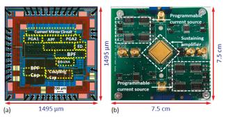
**Figure 4.** (a) Die micrograph of the CMOS sustaining amplifier; (b) Test board used for characterizing the amplifier and integrating with the MEMS resonator to build the oscillator.
