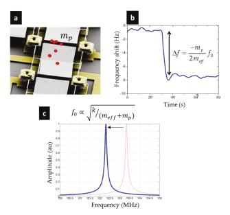
**Figure 1.** The principle of mass measurement (adapted from [28]). (a) Example of a nanoresonator on which particles have landed; (b) Shift in the frequency caused by the arrival of particles. Monitoring in real-time the resonance frequency allows us to deduce the amount of accreted mass; (c) From the spectral perspective: a shift in the spectrum toward low frequencies.
