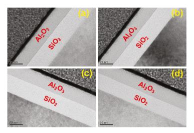
**Figure 5.** Transmission electron microscopy (TEM) images of an atomic layer deposition (ALD)-deposited  $Al_2O_3$  layer (a) before and after (b) 1-min, (c) 5-min and (d) 15-min vapor hydrogen fluoride (HF) etching.
