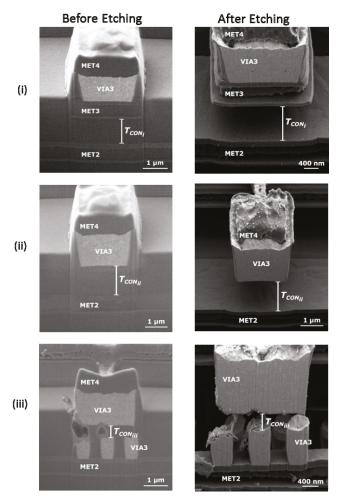
**Figure 3.** SEM images of the cross-section B-B' in Figure 2c over the contact in the three different designs (contact between body relay with different composition and drain) showing before (left images) and after (right images) the releasing: (i) Type I, (ii) Type II and (iii) Type III. These figures can be compared with the cross-section A3-A4 at the contact area of the relay in Figure 1, in which the different composition for contact source and drain are explained.
