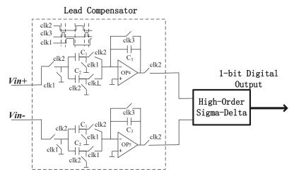
Figure 4. Lead compensator circuit.
