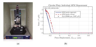
**Figure 14.** Experimental characterization equipment and sample measurement. **(a)** AFM model XE-100 by Park Systems; **(b)** sample contact mode measurement performed on a prototype circular MEMS sensor.
