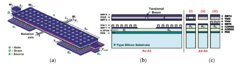
**Figure 1.** (a) 3D schematic of the designed seesaw relay including cross-sectional views (red lines). (b) Cross-section A1–A2 along the length of the relay, the gate electrodes are defined with MET1 and VIA1. (c) Cross-section A3–A4 at the contact area of the relay (between Source and Drain) with the three possibilities: (i) Type I, (ii) Type II, and (iii) Type III.
