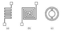
Figure 8. Heater geometries (a) meander, (b) double spiral, (c) drive wheel.
