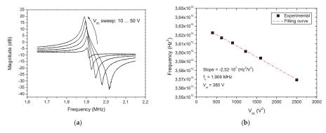
Figure 5. Electrical characterization of the suspended plate resonator with on-chip 0.35- $\mu$ m CMOS readout circuit in open-loop configuration: (a) Measured frequency response (magnitude) for different resonator bias voltages ( $V_{\rm dc}$ ) in air conditions; (b) Plot of the resonance frequency dependency versus the applied bias voltage.
