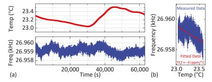
**Figure 8.** (a) Measured temperature variation (top) and fluctuation of oscillation frequency (bottom) for the uncompensated oscillator over 24 h; (b) Linear fit of the oscillation frequency versus temperature.
