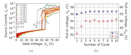
Figure 7. (a) First ten current voltage (I-V) switching characteristics. (b) Evolution of  $V_{PI}$  and  $V_{PO}$  over these ten cycles. Measures correspond to the seesaw relay Type II (W-TiN contact) in ambient conditions.
