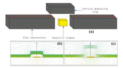
**Figure 5.** (a) The flux modulation micro-structure (b) TMR sensor with flux concentrators and choppers at OFF position (c) The choppers at ON position, the green line represents the size and direction of the magnetic field in the simulation.
