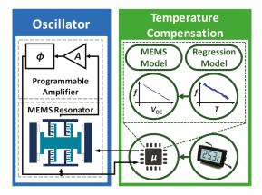
Figure 1. Overview of the temperature-compensated oscillator.
