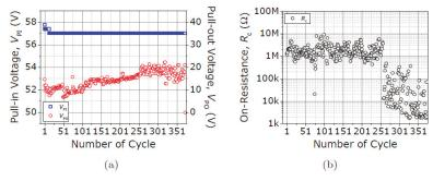
Figure 9. Evolution of (a)  $V_{PI}$ ,  $V_{PO}$  and (b)  $R_c$  over 355 switching cycles under vacuum conditions and  $V_{DS}$  fixed at 3 V. Compliance current set over the measured current level.
