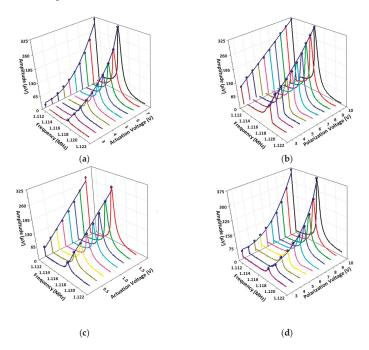
**Figure 7.** Electromechanical response when the frequency is swept around the resonance for different actuation schemes: (a) Amplitude versus f and  $V_{AC}$  for a semitone actuation ( $V_B = 10 \text{ V}$ ); (b) Amplitude versus f and  $V_{B}$  for a semitone actuation ( $V_{AC} = 6.5 \text{ V}$ ); (c) Amplitude versus f and  $V_{AC}$  for a 2f-actuation ( $V_{B} = 10 \text{ V}$ ); (d) Amplitude versus f and  $V_{B}$  for a 2f-actuation ( $V_{AC} = 1.8 \text{ V}$ ).
