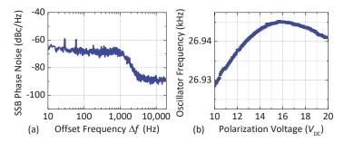
**Figure 6.** (a) Measured single-sideband (SSB) phase noise of the single-crystal SOI MEMS oscillator for  $V_{DC} = 20 \text{ V}$ ; (b) Measured electrical tuning of the oscillator frequency as a function of  $V_{DC}$  (approximately -1 Hz/V for voltages >16 V).
