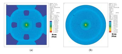
**Figure 17.** ANSYS results for the sensor stress distribution in MPa under an applied concentrated force of  $F_{MAX} = 3 \mu N$  at the top plate center. (a) Square sensor stress distribution; (b) circular sensor stress distribution.
