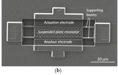
**Figure 4.** Fabricated device in a complementary metal-oxide-semiconductor (CMOS) 0.35- $\mu$ m commercial technology constituted by a plate resonator integrated monolithically with CMOS circuitry: (a) Optical image of the overall CMOS-MEMS oscillator circuit; (b) SEM image of the metal suspended plate resonator.
