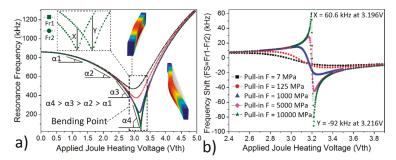
Figure 2. The effect of pull-in force (F) on the (a) Frequency tuning and (b) frequency shift (FS) in COMSOL simulation for Device 1 for a length of 120  $\mu$ m long fixed–fixed beam, where Fr1 and Fr2 are the resonance frequency responses with ambient temperature of Tamb and Tamb + 1 K respectively.
