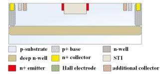
Figure 6. Cross-sectional view of the MMF sensor after the CMOS process.
