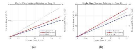
**Figure 8.** Maximum deflection versus central force for a fully clamped circular plate. (a) Analytical model and FE simple model results; (b) analytical model and FE complex model results.
