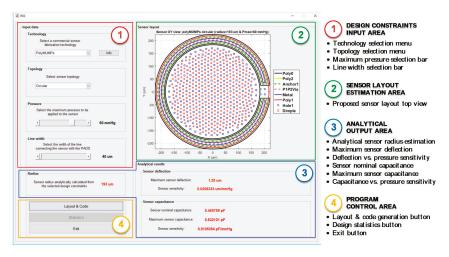
Figure 10. CardioMEMS Design (CMD) main screen, with its working areas and main functionalities displayed.
