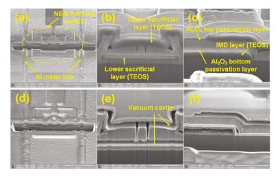
**Figure 4.** (a) Nanoelectromechanical (NEM) memory switch and metal interconnection lines; (b) NEM memory switch and (c) metal interconnection lines before vapor hydrogen fluoride (HF) etching; (d) NEM memory switch and metal interconnection lines; (e) NEM memory switch and (f) metal interconnection lines after vapor HF etching.
