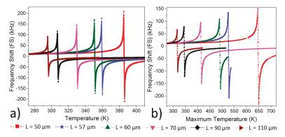
**Figure 4.** Frequency Shift (FS) with respect to 1 Kelvin (K) change by (a) Equation (1), and (b) COMSOL, when length (L) changes from 50  $\mu$ m to 110  $\mu$ m for Device 2 with a device thickness of 1  $\mu$ m.
