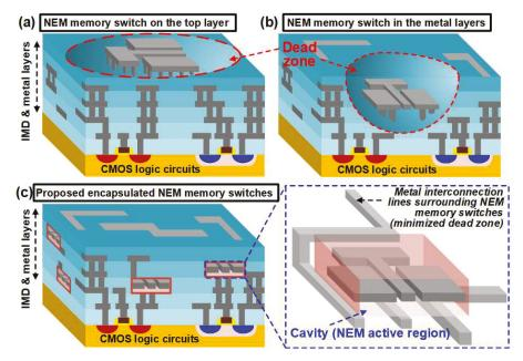
**Figure 1.** Conceptual views of (a) a nanoelectromechanical (NEM) memory switch only on the top layer, (b) a NEM memory switch in the CMOS back-end-of-line (BEOL) metal layers and (c) the proposed encapsulated NEM memory switches for monolithic-three-dimensional (M3D) CMOS–NEM hybrid circuits.
