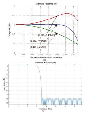
**Figure 9.** (a) Digital decimation filter model (b) Frequency response of first-stage cascade integral comb (CIC) filter (c) Passband amplitude response of CIC before and after compensation (d) Amplitude response of finite impulse response (FIR) low-pass filter.
