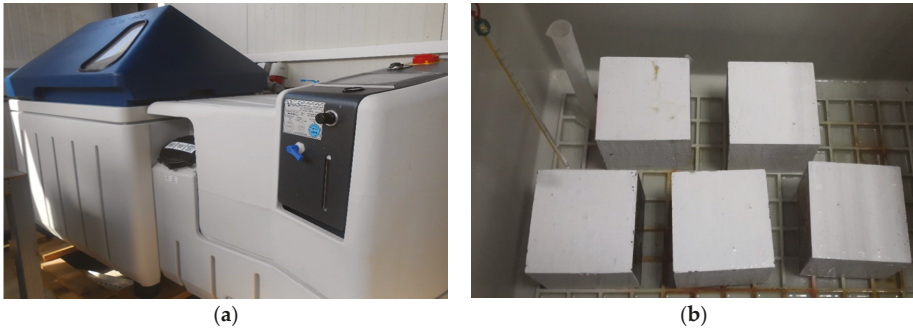
Figure 2. (a) Salt spray chamber and (b) sealed specimens inside the chamber.
