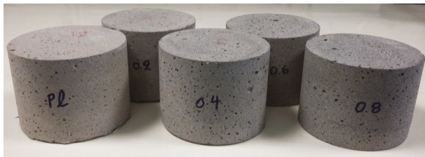
Figure 3. Testing cores drilled off from mortars exposed to accelerated corrosion.
