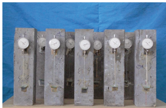
Figure 2. Shrinkage tests of RPC.
