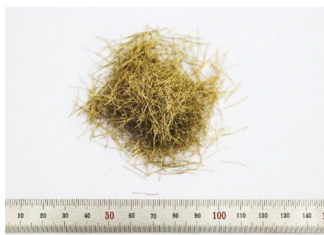
Figure 1. Steel fibre used in this study.
