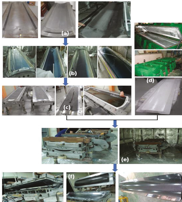
Figure 10. Manufacturing Process of Sandwich cradle; (a) preparing mold & layup of carbon fiber, (b) resin infusion, (c) curing the faces & apply the resin evenly, (d) prepared core, (e) inserting core into molds and curing/bonding, (f) de-molding and hole machining.
