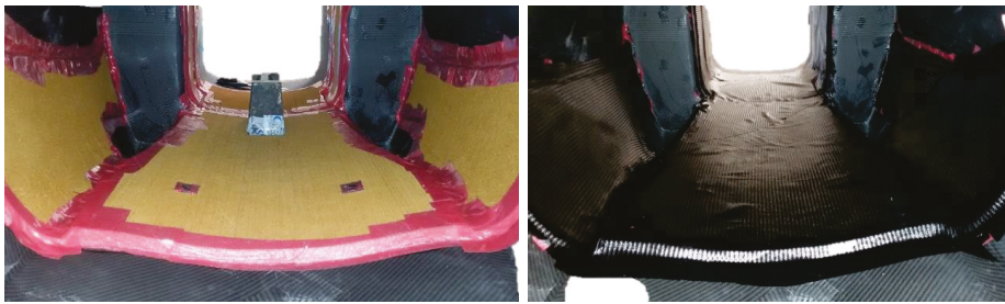
Figure 13. Second lamination in the central part: Nomex honeycomb (left) and composite layers (right).
