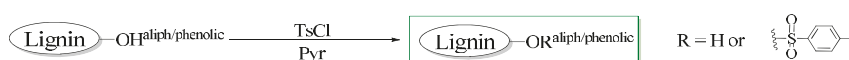
Figure 1. Reaction scheme for synthesizing tosylated lignin. Abbreviations: -\text{OH}^{\text{aliph}} —aliphatic hydroxyl groups in lignin ( 1.65 \text{ mmol g}^{-1} as determined by ^{31}\text{P} -NMR measurement); -\text{OH}^{\text{phenolic}} —phenolic hydroxyl groups in lignin ( 2.12 \text{ mmol g}^{-1} as determined by ^{31}\text{P} -NMR measurement); TsCl—tosyl chloride; and Pyr—pyridine.
