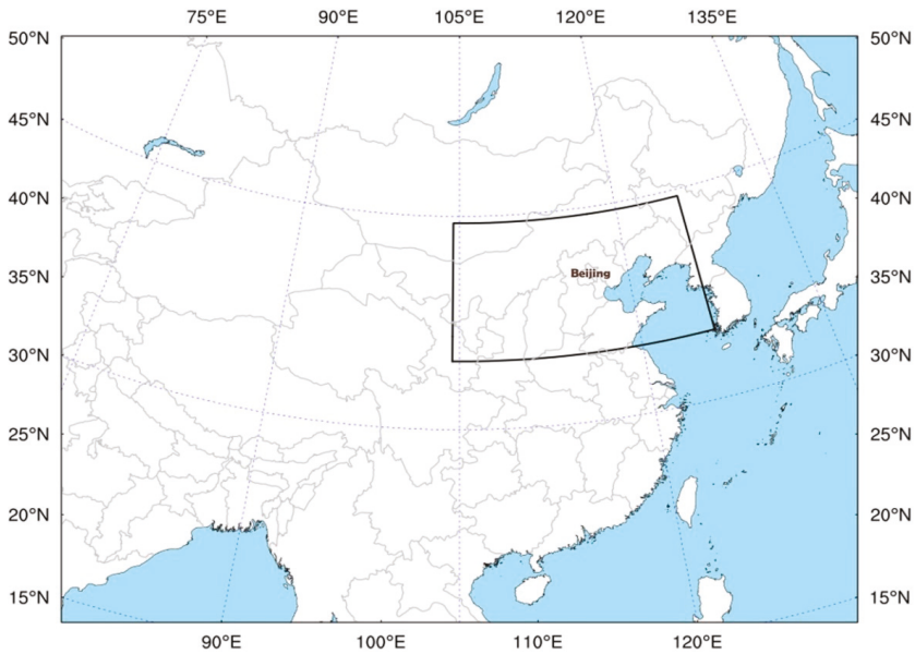
Figure 1. Two nested domains in the RMAPS (Rapid-Refresh Multi-Scale Analysis and Prediction system). The outside box is a 9 km horizontal resolution domain, the inside black box represents a 3-km horizontal resolution domain that is centered in Beijing.
