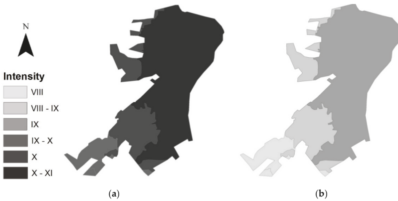
Figure 3. Intensity map for the city of Imzouren including soil effects according to (a) the deterministic scenario and (b) the probabilistic scenario.
