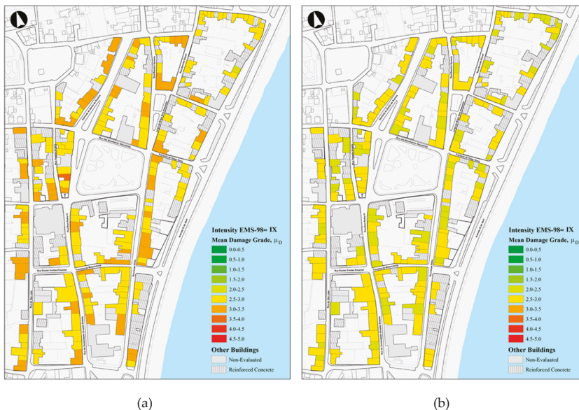
Figure 3. Mapping of damage scenarios for the old city centre of Horta: (a) before and (b) after the application of seismic retrofitting strategies, adapted from Ferreira et al. [30].
