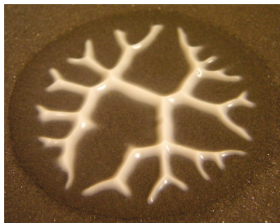
Figure 3. Fingering aspect of the remaining deposit of yield stress fluid after separation of two plates initially squeezing a thin fluid layer. (Photo Q. Barral).
