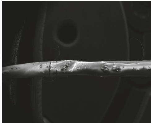
Figure 3. Electron micrograph of a dextran coated Parylene-C neural probe. A crack can be seen on the left-hand side of the probe which was formed after buckling. Reproduced with permission from [31]; published by IOPscience, 2017.
