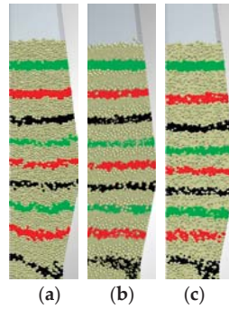
Figure 4. Internal wall of solid flow under three burden layer conditions simulated by the sector model 1 via DEM, i.e., full coke (a), layered coke and ore pellet (b) and mixed coke and ore pellet (c).
