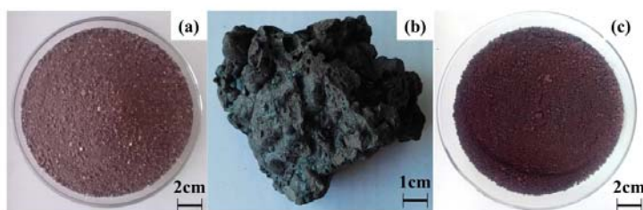
Figure 1. Experimental material (a) stainless steel dust (SSD) (b) stainless steel slag (SSS) (c) \text{Fe}_2\text{O}_3 .
