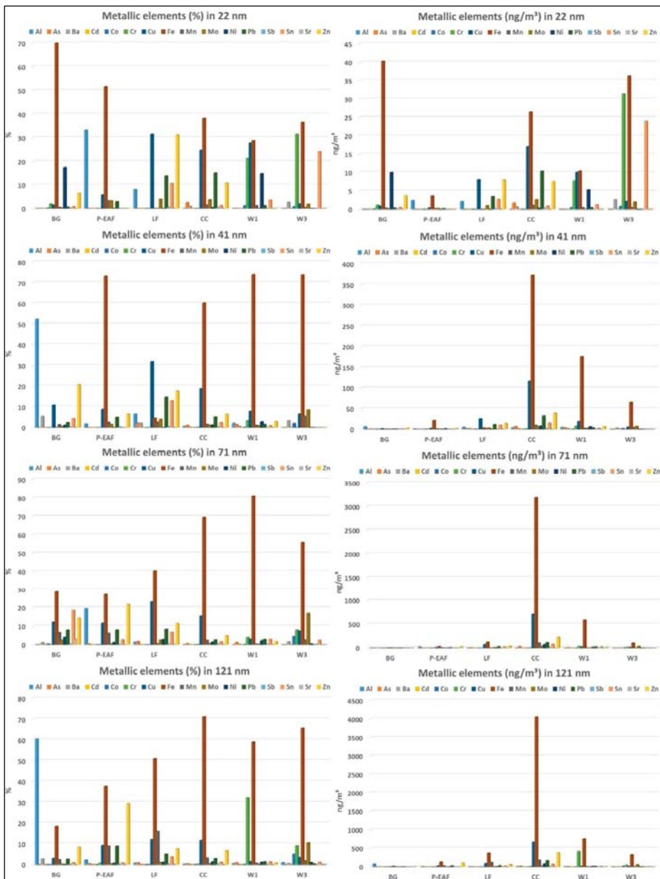
Figure 6. Distribution of the metallic elements (percentage value (left) and \text{ng}/\text{m}^3 (right) for each fraction) in the different UFP size ranges collected by ELPI+, for each area and working station. The percentages shown in the figure represent the fraction of each metallic element on the total of the metallic elements determined in each size range for each sampling site.
