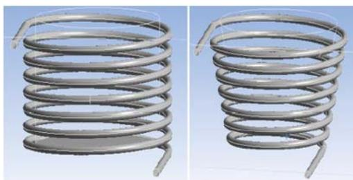
**Figure 6.** Generic cylindrical and conical configuration of conformal cooling channels.
