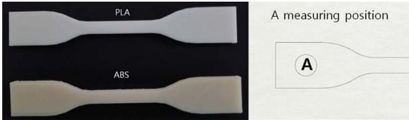
**Figure 2.** Polylactic acid (PLA) and acrylonitrile butadiene styrene (ABS) specimens fabricated by 3D printers and the measuring position for the Fourier transform infrared (FTIR) method.
