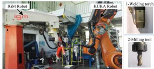
Figure 2. Two-robot cooperative platform for implementing HWMP.
