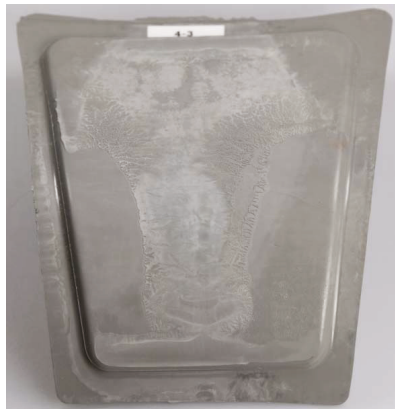
Figure 5. Formed hybrid laminates with sensor functionality at preheating temperature 200 °C and tool temperature 170 °C.
