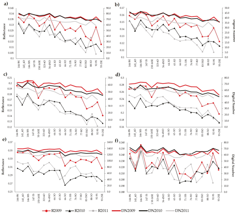
Figure 3. Spectral signature average expressed as reflectance and the digital number for each quadrant ((a) band1, (b) band2, (c) band3; (d) band4, (e) band5, (f) band7).
