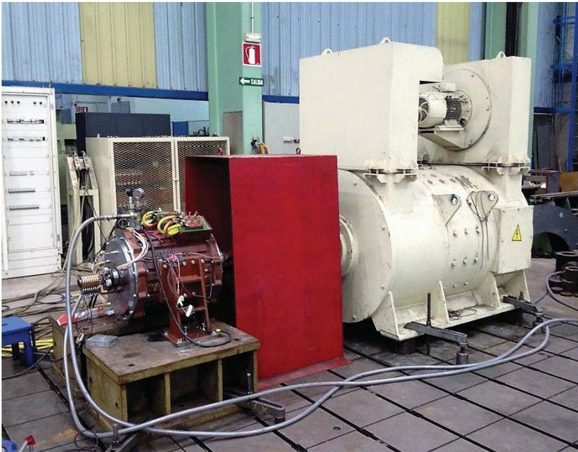
Figure 15. IPMSM Prototype at test bench.
