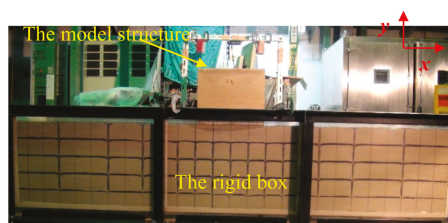
Figure 1. Shaking table with experimental set up.
