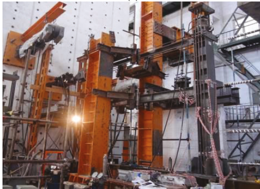
Figure 11. The physical substructure test model of the steel frame structure: (a) the design drawing of the physical substructure test model; and (b) the manufactured test model at the lab.
