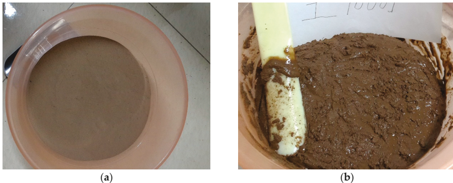
Figure 1. Viscous fluid composition: (a) silt; (b) mixture of methyl silicone oil and silt.
