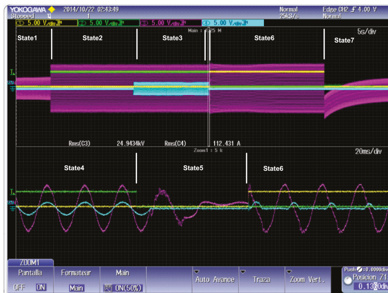
Figure 11. HST travelling at 280 km/h from section 2 to section 1. Ch1, S1 command; Ch2, S2 command; Ch3, NS voltage; Ch4, NS current.
