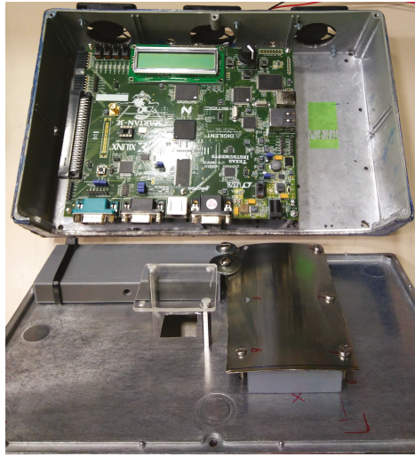
Figure 2. Shielding of the PCB attached to the cover of the filter box.
