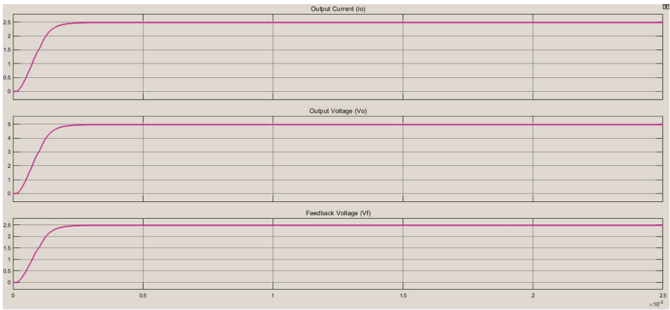
Figure 6. Converter output voltage and current during HIL simulation for the case V_i = 16\text{ V} and R_{load} = 2\ \Omega without fault emulation.
