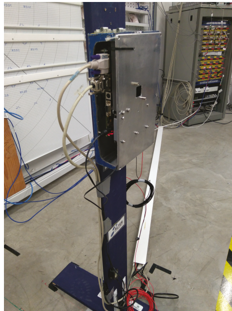
Figure 5. Filter Box with the PCB (and DUT) inside and the connections to the different ports and power supply.
