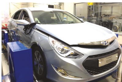
Figure 1. TMED type parallel hybrid vehicle and chassis dynamometer.
