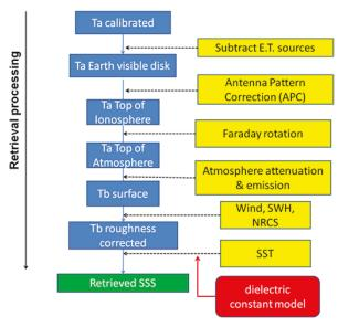
**Figure 5.** Flow diagram illustrating the steps in the Aquarius salinity retrieval algorithm. The process starts at the top with calibrated antenna temperature, TA, from the radiometer and ends with a measurement of SSS at the surface.
