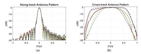
**Figure 3.** The antenna pattern of the eight-element prototype of the 1D IMI, including the along-track and cross-track antenna patterns in (a) and (b), respectively.
