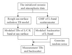
Figure 3. The simplified flow chart of the simulation process for measurements of MICAP.
