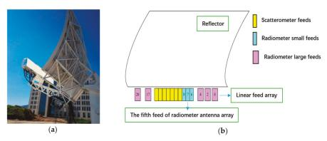
**Figure 2.** A ground-based prototype of the one-dimensional interferometric microwave imager (IMI). (a) Photo of the ground-based IMI prototype. (b) Arrangement of the small and large antenna units in the feed array of the IMI prototype.
