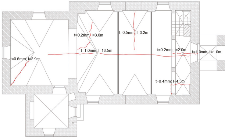
Figure 4. Registered crack pattern of analysed barrel vault before rehabilitation in 2013 [6].
