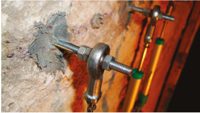
Figure 12. Displacement transducers attached to the wall.
