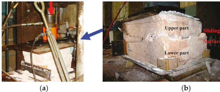
Figure 10. (a). Short stone masonry specimen subjected to sliding shear; (b) Sliding mode of failure of short stone masonry specimen.
