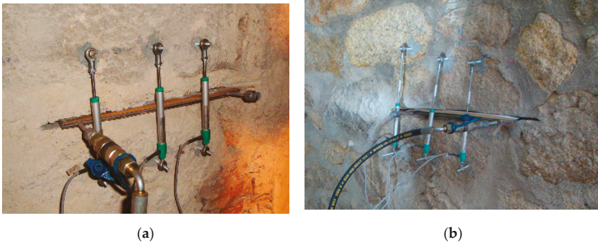
Figure 13. Single flat-jack testing: (a) conducted in the Órfeão de Viseu and (b) in the Águas de Viseu (b).
