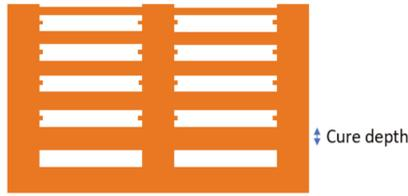
Figure A1. Bridge structure illustration for cure depth measurement.
