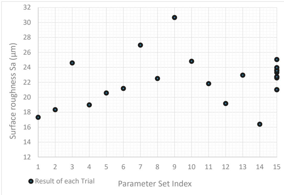
Figure 7. Replicate plot for 35° down-facing surfaces: Surface roughness (*Sa*) for each trial number.
