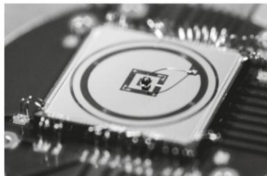
**Figure 15.** Opto-ASIC mounted onto PCB with assembled laser diode on the additional metal top layer, in comparison to Figure 12.
