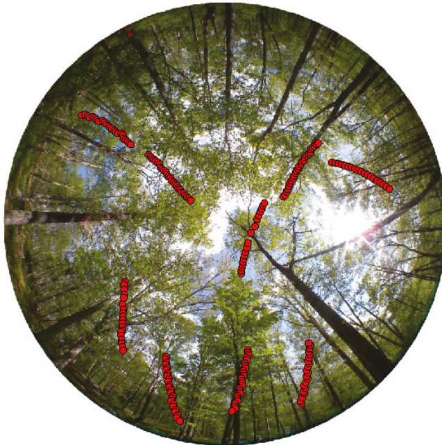
Figure 2. A hemispherical sky-oriented photo taken during the spring data collection at West Point, New York, with the global positioning system (GPS) satellite vehicle positions (red circles) plotted inside the image.
