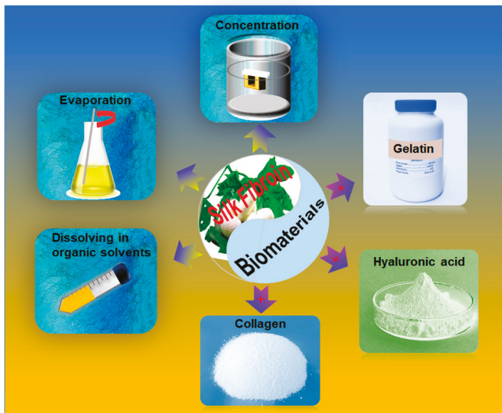
Figure 2. Schematic of methods to optimizing the rheology of SF bioink. SF is a biomaterial with impressive biocompatibility and mechanical properties. As a bioink, its rheology should be adjusted in aqueous system by different strategies. The gradient arrow without “+” indicated that their rheology could be regulated by concentration, evaporation, and dissolving in organic solvents; the arrow with “+” shows that SF solutions were combined with other biopolymers, such as collagen, hyaluronic acid, and gelatin, respectively, to enhance their rheology.
