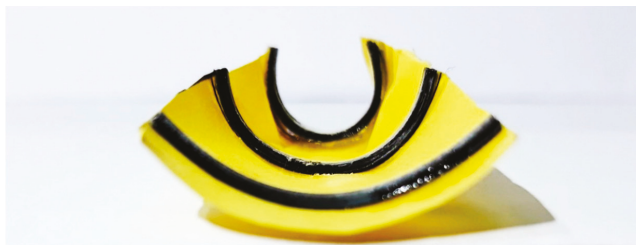
Figure 9. Configuration of the flat sheet reinforced by three straight 4D-printed beams after the heating–cooling process.
