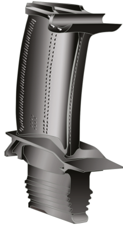
Figure 1. Illustration of a high-pressure turbine blade [8]. The internal channels create a protective layer of cool air to protect the outer surface of the blade.
