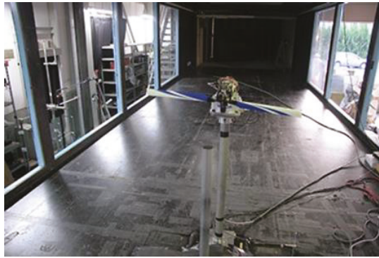
Figure 4. Test model and dummy tower installed in the wind tunnel.
