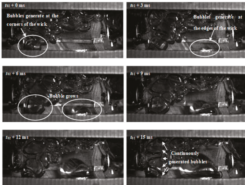
Figure 11. Evolution of vapor–liquid two-phase flow inside the wick thermosyphon ( H = 15 mm, \varphi = 50\% , q = 20 W/cm^2 ).
