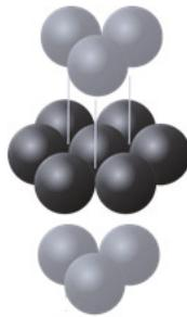
**Figure 4.** Formation of a hexagonal closest packed (HCP) crystal.
