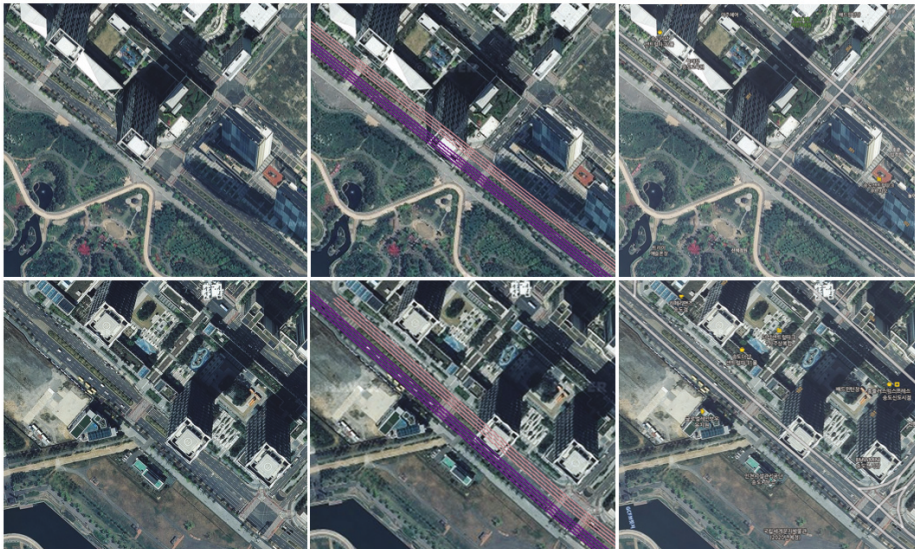
Figure 6. More results of the detected road lanes on Route 2 are accumulated to generate a lane-level digital map with the help of a GPS/INS sensor. The left column shows the satellite images, the middle column the resulting lane-level map overlapped with the satellite images and the right column the existing road-level map provided by Naver Map [41].
