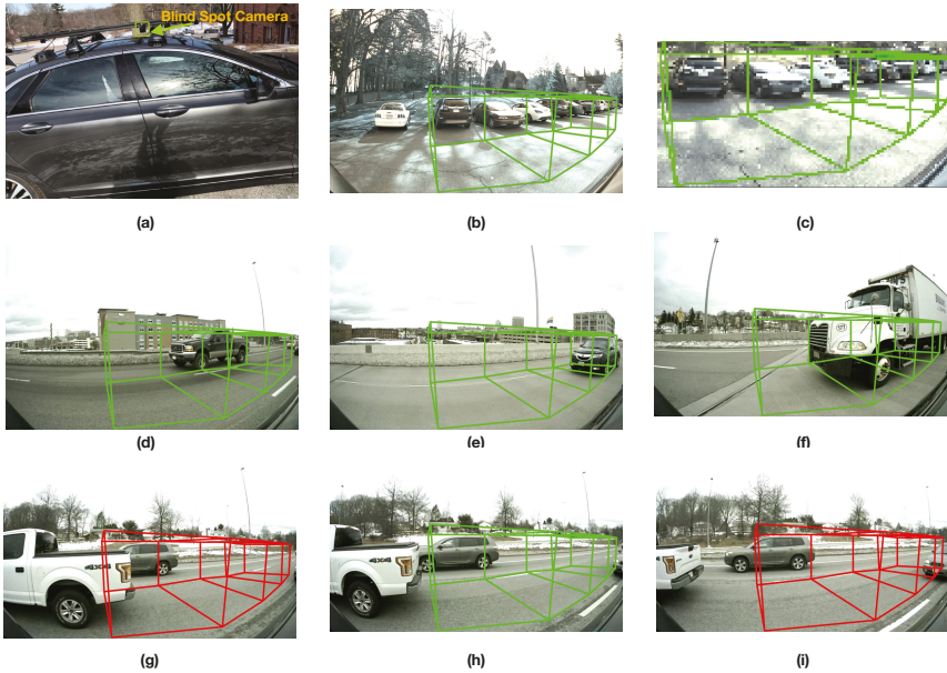
Figure 5. We show the position of our camera in (a). (b) is the blind spot region in the view of camera. (c) is the training image after preprocessing (b). (d) is an example of No-Car class in training data, (e,f) are examples of Car class in training data. (g–i) are examples of the final output of our blind spot detection system. If the model finds a car, it will alarm the driver by changing the color of the box. Our model is fairly accurate and can exactly account for the blind spot region.
