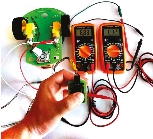
Figure 9. Electric power delivered to one of the wheels when p = 1 and the joystick is displaced completely in the positive direction of the X-axis.
