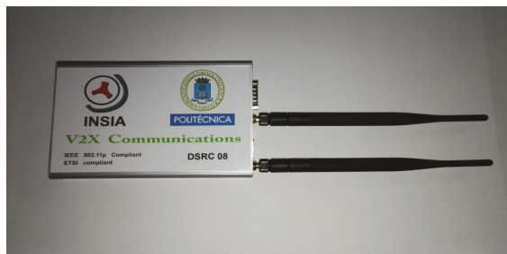
Figure 1. DSRC INSIA-V2X (Dedicated Short-Range Communications) module.
