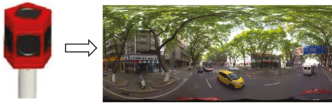
Figure 3. The multi-camera panoramic vision system and the acquired panoramic image.
