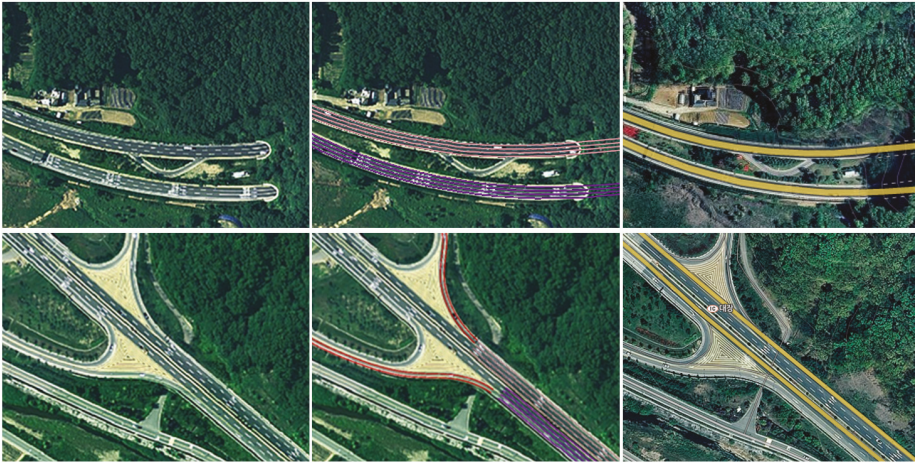
Figure 5. Detected road lanes on Route 1 are accumulated to build a lane-level digital map with the help of a GPS/INS sensor. The left column shows the satellite images, the middle column the resulting lane-level map overlapped with the satellite images and the right column the existing road-level map provided by Naver Map [41].
