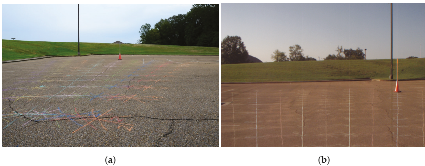
Figure 7. (a) Markings on the ground. (b) View from the camera. Markings on the ground covering the full FOV and detection range of the camera.
