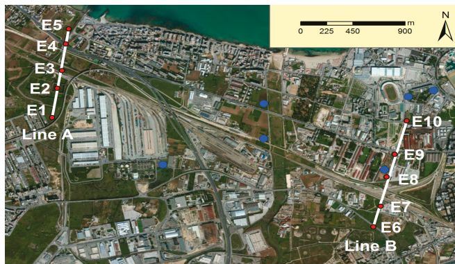
Figure 3. ERT profile locations. Blue points are boreholes (six) used for salinity measurements to calibrate Equation (7) by using resistivity data provided by ERT profiles.
