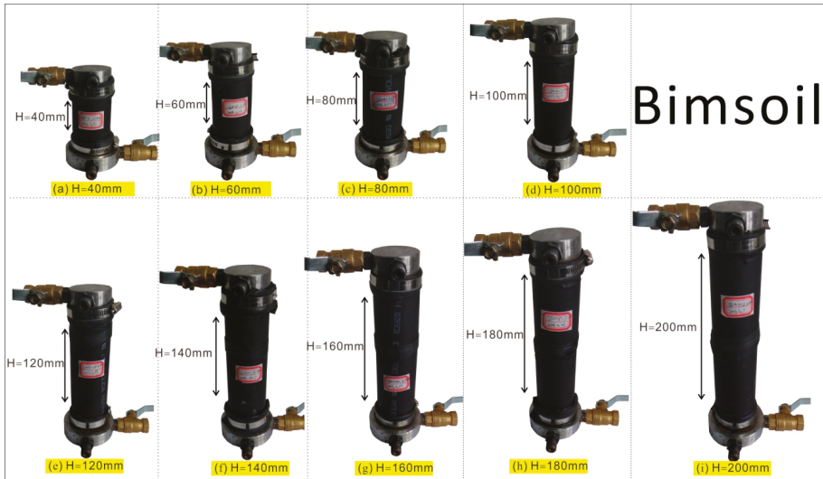
Figure 3. The sample chamber system for bimsoil samples with different height, taking samples with RBP (rock block percentages) of 30% as an example.
