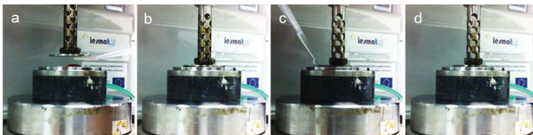
Figure 2. Image sequence of the gel filling process on the rheometer. Once the sample was mixed, it was pipetted in situ onto the rheometer plate (a); then, the gap was adjusted (b), and the sample was covered with oil (c) to prevent evaporation; the set-up was then ready to conduct the experiment (d).
