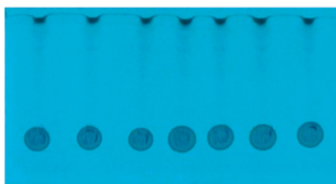
Figure 5. The serum sample chromatograms after development using SPK3 procedure; stationary phase: HPTLC Silica gel 60 F254 (Merck), mobile phase: methanol.
