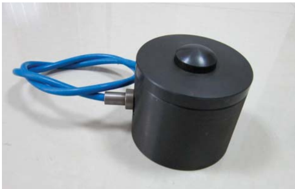
(c) The MA60 backfill stress meter.
