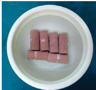
Figure 3. Testing water absorption rate.
