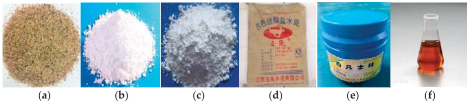
Figure 1. The raw materials of similar-material: (a) River sand; (b) Calcium carbonate; (c) Talc powder; (d) White cement; (e) Vaseline; (f) Antiwear hydraulic oil.
