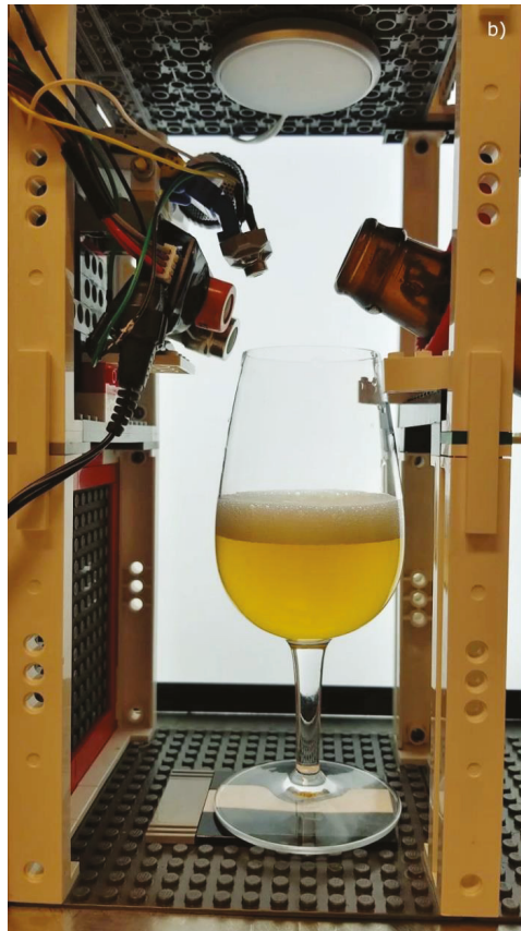
Figure 1. Equipment used to assess beers physical measurements; (a) robotic pourer, RoboBEER, which was used to assess the color and foam-related parameters and (b) a frame of a video taken to analyze the beer using computer vision algorithms.
