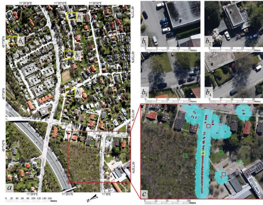
Figure 10. (a) A typical frame from the training sample. (b 1 ~ b 4 ) Typical difficult detection cases. (c) The close-to-vehicle region (shaded blue) and categorical sampling positions.
