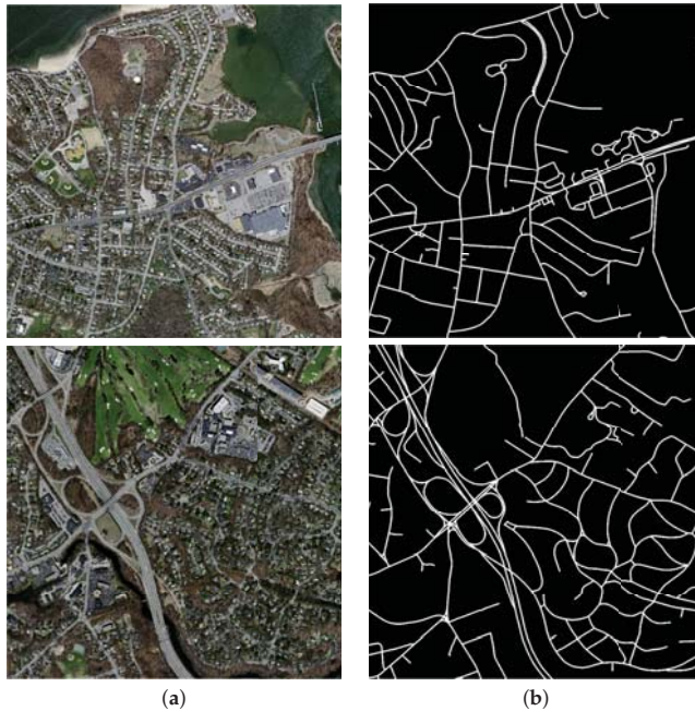
Figure 4. Two sample aerial images from the Massachusetts road corpus, where a row refers to each image (a) Aerial image and (b) Binary map, which is a ground truth image denoting the location of roads.
