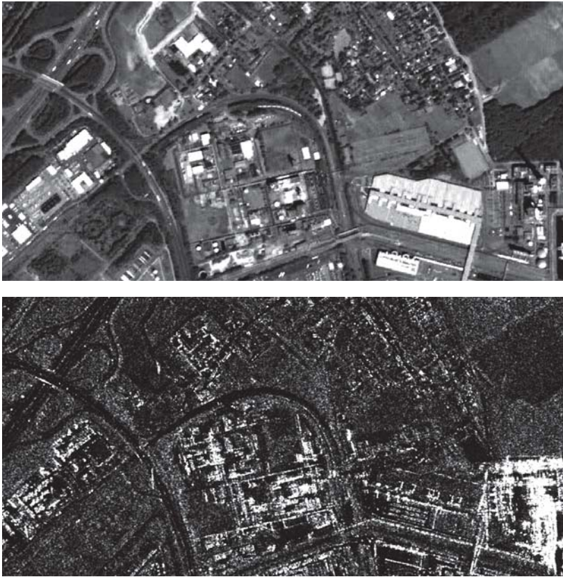
Figure 1. Visual comparison of an optical ( top ) and SAR image ( bottom ) acquired over the same area. Both images have a ground sampling distance of 1.25 m.
