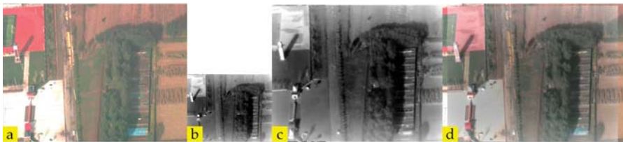
Figure 14. Third experiment of scale calculation: (a) original image; (b) original infrared image; (c) scale-transformed result of image (b); and (d) fusion image of images (a) and (c).
