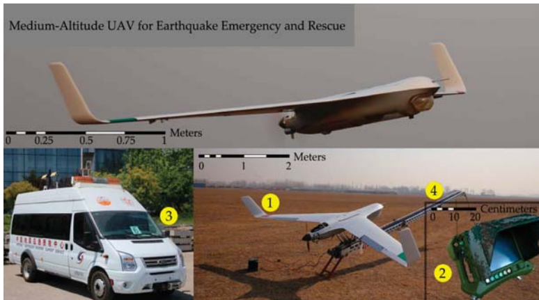
Figure 1. UAV system for earthquake emergency and rescue including: (1) unmanned aerial vehicle (UAV); (2) ground control system; (3) information processing center; and (4) launcher.
