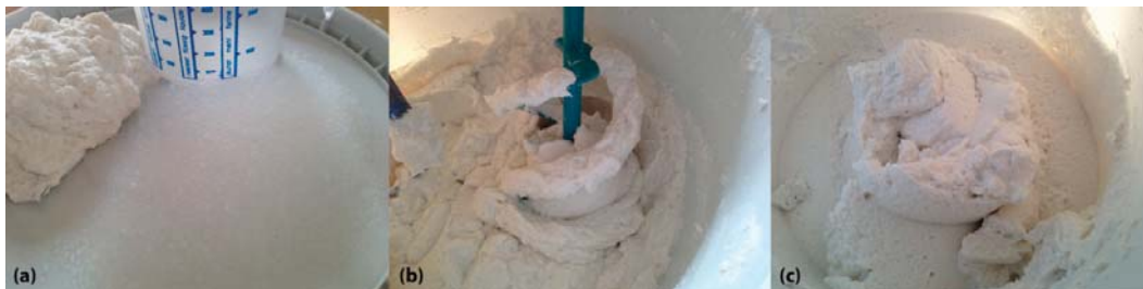
Figure 1. Various steps of the mixing: (a) original components; (b) mixing phase; (c) final composition of the plaster.
