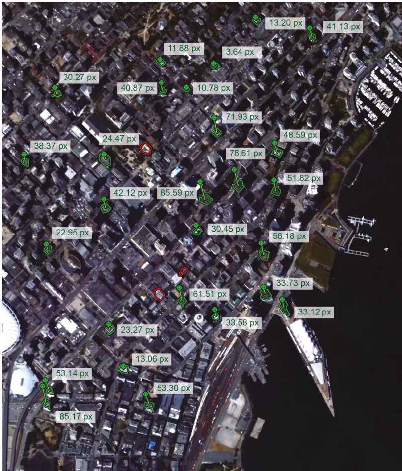
Figure 4. Radial displacement of building rooftops in pixels, measured by tracking the movement of rooftop outlines over the course of the video. Initial building rooftop outlines appear as green polygons. Green targets represent the centroids of the tracked outlines' final positions. Green vectors represent the radial displacement of the outlines. Red polygons represent three buildings that were lost during the tracking progress.
