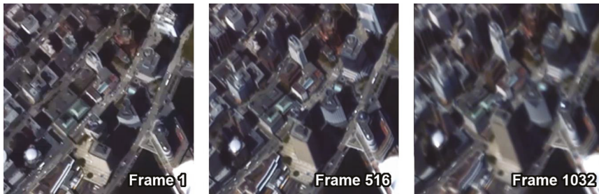
Figure 1. Example of radial displacement of buildings over the course of a high definition video from space.
