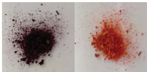
Figure 9. Colour change of fac -[Fe(4-ima-Bp) 3 ](ClO 4 ) 2 ·3MeOH 1 heating from 298 K (left) to 423 K (right).
