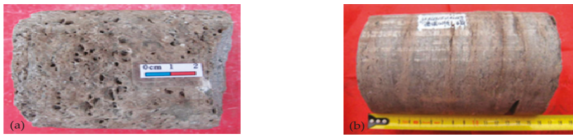
Figure 2. Core samples from the carbonate gas reservoir of Anyue gas field. (a) Core sample with vugs and pores; (b) Core sample with micro fractures.
