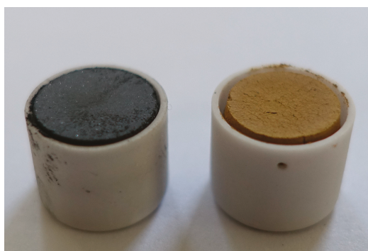
Figure 2. The appearance of char sample before and after gasification at 1273 K for 99 min.
