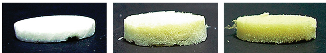
Figure 7. Appearance of (left) n-cellulose, (middle) n-chitin, (right) n-cellulose + n-chitin + sericin. The latter contains glutaraldehyde. Reprinted with permission. Copyright © 2014 Elsevier [184].
