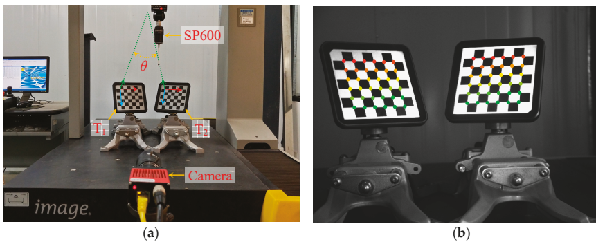
Figure 13. Experiment for measuring attitude. (a) Determining \theta via CMM and camera. (b) One shot in 15 trials with located corners.
