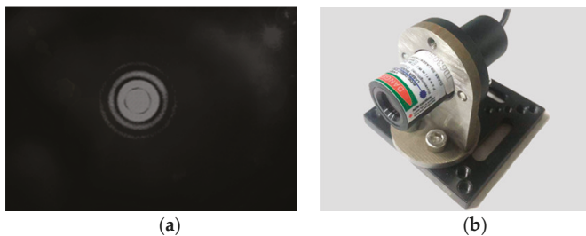
Figure 25. (a) Laser spot image in 70 m receiving distance; (b) high power laser with optical lens.
