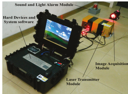
Figure 5. Main composition of the real-time tunnel deformation monitoring system.
