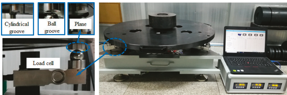
Figure 13. Experiment platform for measuring mass and CG.
